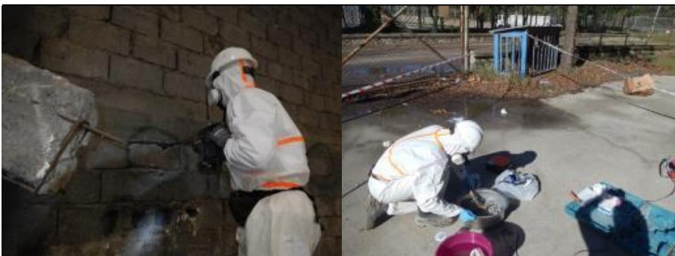
**Figure 5.6 Collection of building blocks (left) Outside processing of blocks prior to transfer to laboratory (right)**
